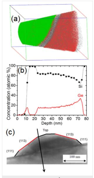
**Figure 9:** (a) APT volume  $(90 \times 90 \times 130 \text{ nm}^3)$  and (b) Si and Ge 1D concentration profiles measured in (a). Figure 9c indicates the direction in which the concentration profiles were measured in the island.
