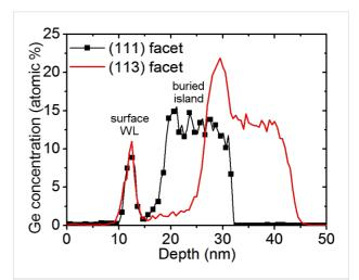
**Figure 7:** Top-down 1D Ge concentration profiles measured in two different APT volumes, one in the direction perpendicular to a (111) facet (black solid squares), and the other in the direction perpendicular to a (113) facet (red solid line).
