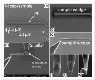
Figure 1: SEM images acquired during APT sample preparation in a dual-beam FIB process. The image sequence (a to f) corresponds to the chronological steps required for the fabrication of an APT tip.
