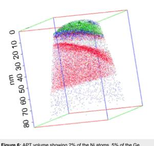
**Figure 6:** APT volume showing 2% of the Ni atoms, 5% of the Ge atoms, and 100% of the O atoms (the Si atoms are not shown). The O atoms detected in the bulk of the sample are actually due to noise.
