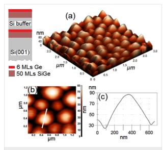
**Figure 2:** Sketch of the sample structure and AFM measurements performed on the sample surface after MBE growth: (a)  $3 \times 3 \ \mu m^2 \ 3D$  image, b) 2D image, and c) height variations measured along the white line in (b).
