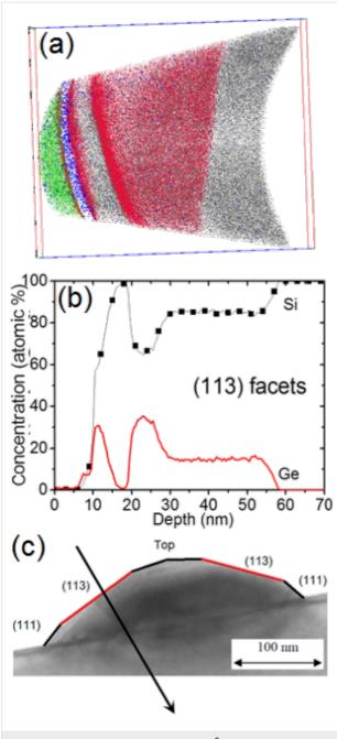
**Figure 10:** (a) APT volume  $(70 \times 70 \times 85 \text{ nm}^3)$  and (b) Si and Ge 1D concentration profiles measured in this volume. Figure 10c indicates the direction in which the concentration profiles were measured in the island.
