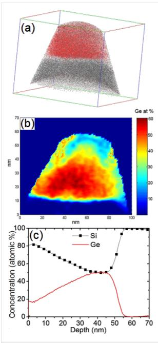
Figure 8: APT analysis: (a) 3D volume (120 × 120 × 100 nm³), (b) 2D map of the Ge concentration distribution in the center of the volume presented in Figure 8a, and (c) top-down 1D Si and Ge concentration profiles measured in the volume presented in Figure 8a.
