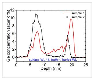
**Figure 4:** Top-down, 1D Ge concentration profiles measured between the islands in two different samples. The profiles go through the surface WL, the Si buffer, the buried WL, and end in the Si substrate.
