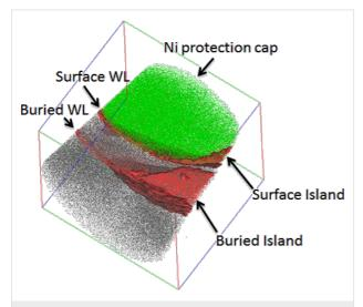
Figure 3: APT volume ( $100 \times 100 \times 90 \text{ nm}^3$ ) obtained from the sample. Green, gray, red and blue dots correspond to Ni, Si, Ge and O atoms, respectively. 2 atom % Ge isoconcentration surfaces are also shown (dark red surfaces).
