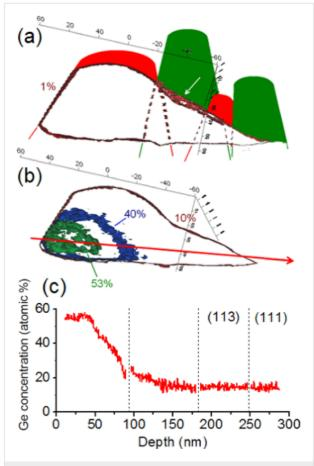
**Figure 11:** APT measurements obtained for four APT volumes (green and red surfaces) which form almost half of a Ge island: (a) Ge isoconcentration surface of 1 atom %, (b) Ge isoconcentration surfaces of 53, 40 and 10 atom %, and (c) Ge 1D concentration profile measured in the direction indicated by the red arrow in (b).
