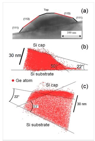
**Figure 5:** Cross-sectional TEM image of a typical dome island (a), and side-views of two different APT volumes showing only the Ge atoms they contain (b and c).
