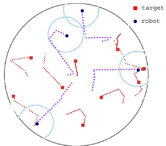
Fig. 2. Bounded arena, with 4 robots moving randomly (circle). The radius of the arena is 5, the radius of the sensory perception range of the robots is 1. There are 9 targets (square), also randomly moving. The dotted lines indicate the paths followed by the robots and the targets. The targets have different speeds: the closer the dots, the lower the speed.
