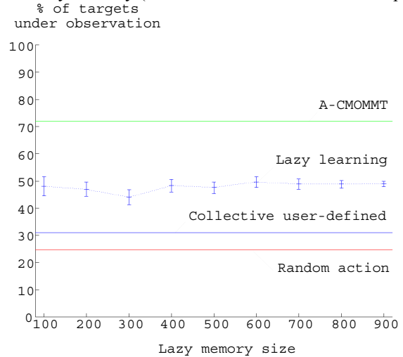
Fig. 9. Performances of the cooperative lazy (Q-)learning compared to a random action selection policy, a user-defined non cooperative policy and A-CMOMMT. The size of the lazy memory varies between 100 to 900 situation-action pairs. There are 10 robots and 10 randomly moving targets. The results are the mean of 10 different experiments per point for lazy learning policy, and 100 experiments for the other 3 policies. Each experiment duration is 1000 iterations.
