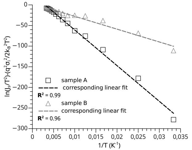
**Figure 4.** Richardson modified plots and corresponding linear fits for Mn<sub>5</sub>Ge<sub>3</sub>C<sub>0.6</sub>/Ge(111) Schottky contacts with and without a  $\delta$ -doped layer according to a multi-Gaussian distributions model of the SBH.
