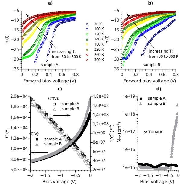
**Figure 2.** a) and b) typical forward current-voltage characteristics for Schottky diodes without (sample A) and with (sample B) a δ-doped layer, c) C-V and  $1/C^2$ -V typical plots at 160 K and 1 MHz and d) corresponding numerically extracted capacitance-voltage profiles  $N_{CV}$ .
