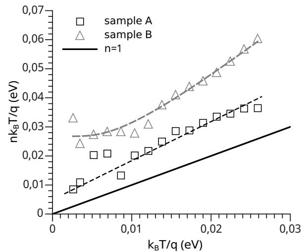
**Figure 5.** Plots of  $\frac{nk_B T}{q}$  vs  $\frac{k_B T}{q}$  for the sample with and without the  $\delta$ -doped layer. The plain dark line corresponds to an ideal Schottky barrier following the TE theory with an ideality factor  $n=1$ . The dotted lines correspond to the fits of the experimental data according to the appropriate models (cf. table 3).
