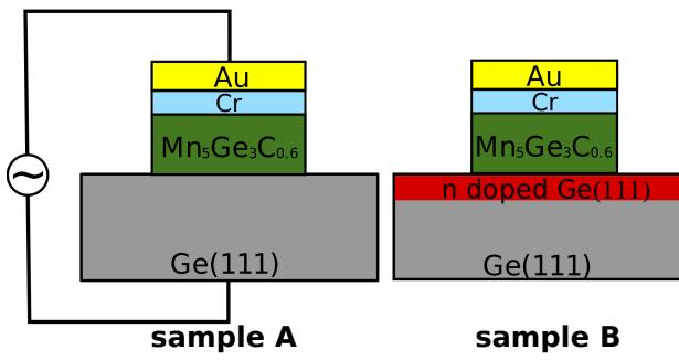
**Figure 1.** Drawings of the investigated Schottky diodes with the P δ-doped layer on the right and without on the left.
