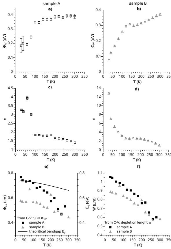
**Figure 3.** a) and b) Schottky barrier heights  $\Phi_{IV}$  of the samples without (A) and with (B) a  $\delta$ -doped layer respectively, c) and d) ideality factors  $n$  from the I-V measurements. e) Schottky barrier heights  $\Phi_{CV}$  from the C-V measurements and f) depletion length  $W$  in micrometer calculated from the C-V curves on samples without and with a  $\delta$ -doped layer.
