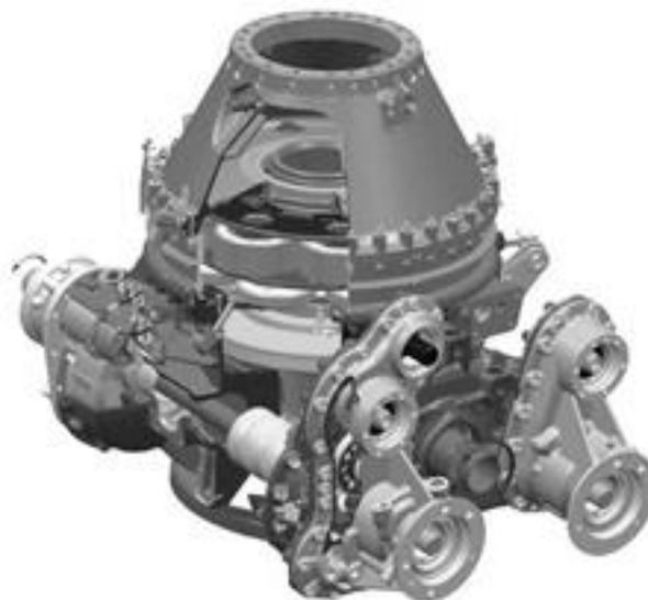
Fig. 1. View of a helicopter main gearbox.
