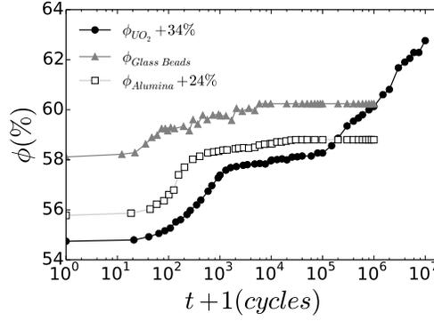
Figure 1: Examples of experimental results under horizontal vibrations at 100 Hz and 7g acceleration. The tank was  $15 \times 15$  mm<sup>2</sup>.
