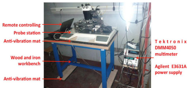
Figure 5. Picture of the proposed test bench, embedded in the low-noise environment.
