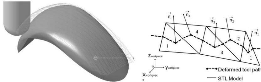
Figure 4: Discontinuities observed on the deformed tool path.
