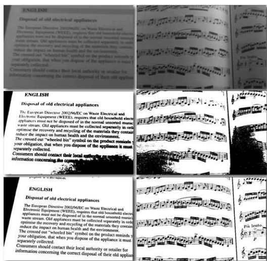
Fig. 10. Binarization of live images using a smartphone. (top) Grey input, (middle) Otsu's method, (bottom) proposed method.
