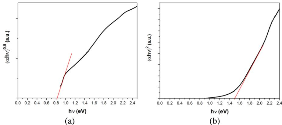
**Fig. 12.** Dependence of (a)  $(\alpha hv)^{0.5}$  and (b)  $(\alpha hv)^2$  on photon energy  $h\nu$  plot for famatinite NCs based 100 nm thick film
