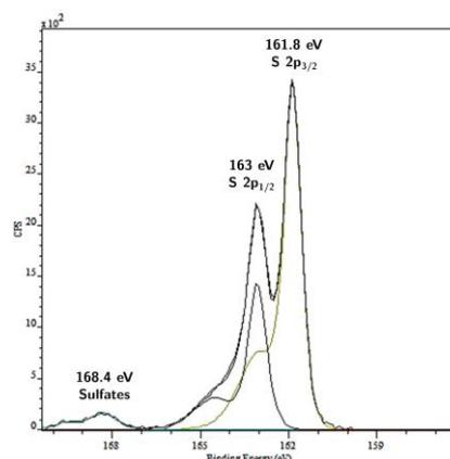
**Fig. 7.** XPS S 2p spectrum of famatinite NCs
