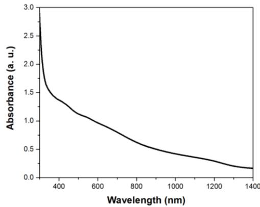
**Fig. 11.** UV/VIS/NIR absorption spectrum of famatinite NCs based 100 nm thick film
