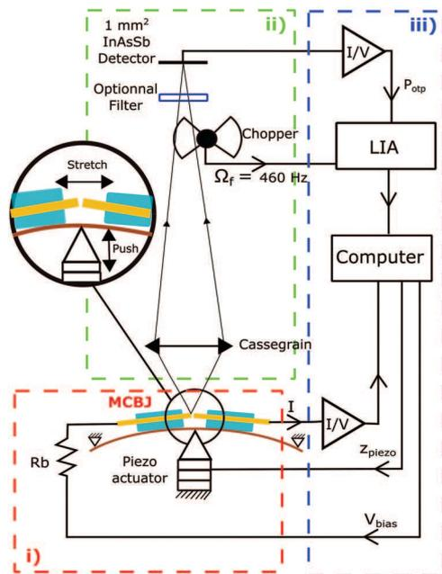
Fig. 1: (Colour online) Experimental set-up. i) MCBJ with a piezo actuator. Photons are collected using a reflective Cassegrain objective ( $15\times$ ,  $\text{NA} = 0.5$ ), optionally filtered and chopped at 460 Hz and detected using a cooled InAsSb IR detector. ii) The magnified view shows the MCBJ principle (push-to-stretch movement). The control and acquisition electronics consists of a current-voltage converters, a lock-in amplifier (LIA) and a computer.
