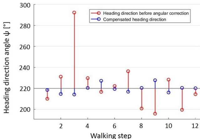
Fig. 6. Evolution of the measured heading direction angle  $\psi$  before (in red) and after (in blue) angular correction using only the UV-polarized light compass during a straight-forward walking task. Walking steps measurements from 1 to 6 were acquired on 02/18/2017 while the next six measurements were acquired on 02/20/2017.
