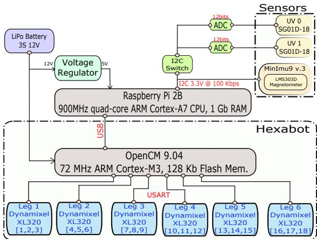
Fig. 4. Robot electronic architecture. The dashed line marks out the robot controller and actuators. The magnetometer and UV-polarized light sensors (in yellow) are connected to the Raspberry Pi 2B board using I2C communication protocol.
