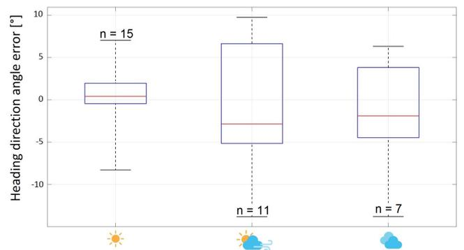
Fig. 5. Heading direction angle errors in degrees in function of weather conditions. From left to right, the median heading direction angle error measured is equal to  $0.4^{\circ}$ ,  $-2.9^{\circ}$ , and  $-1.9^{\circ}$ . UV-index from 1 to 2 (source: French Meteorological services).
