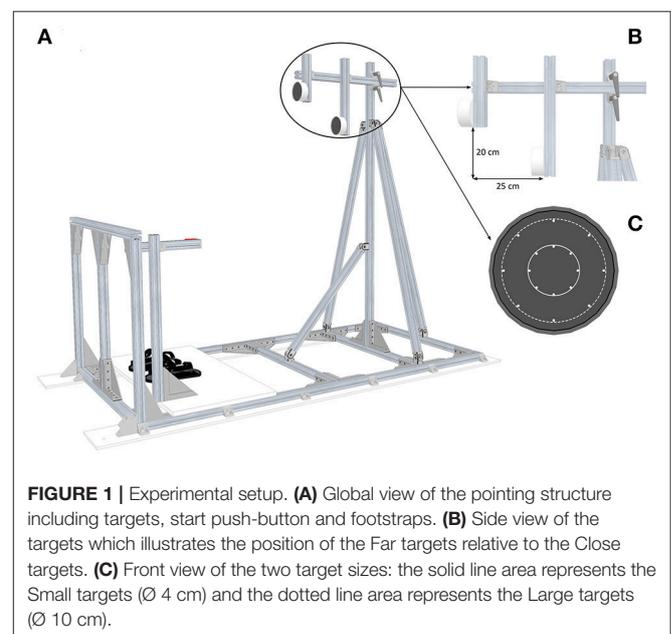
**FIGURE 1** | Experimental setup. (A) Global view of the pointing structure including targets, start push-button and footstraps. (B) Side view of the targets which illustrates the position of the Far targets relative to the Close targets. (C) Front view of the two target sizes: the solid line area represents the Small targets ( $\varnothing$  4 cm) and the dotted line area represents the Large targets ( $\varnothing$  10 cm).
