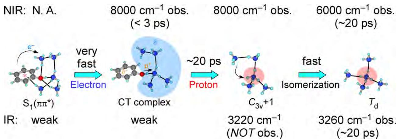
**Figure 3** Structures and responsible absorption features (upper side: electronic transitions in the NIR region, lower side: NH stretching transitions in the 3  $\mu\text{m}$  region) of the PhOH-(NH<sub>3</sub>)<sub>5</sub> cluster and the  $\bullet\text{H}(\text{NH}_3)_5$  product along the course of the decoupled ESHT reaction mechanism.
