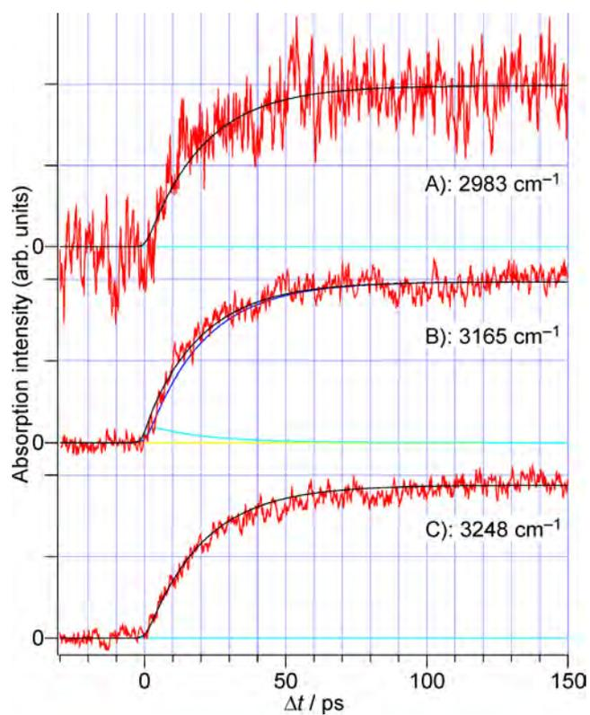
**Figure 7** Time evolutions of transient NH stretching vibrations of PhOH-(NH<sub>3</sub>)<sub>5</sub> after the  $\pi\pi^*$  excitation probed at A) 2983 cm<sup>-1</sup>, B) 3165 cm<sup>-1</sup>, and C) 3248 cm<sup>-1</sup>, respectively. Best fitted curves and population decomposition are also presented with the same format as in Figure 5. In A) and C) the best fitted curves completely overlap on contribution from the  $T_d$  isomer.
