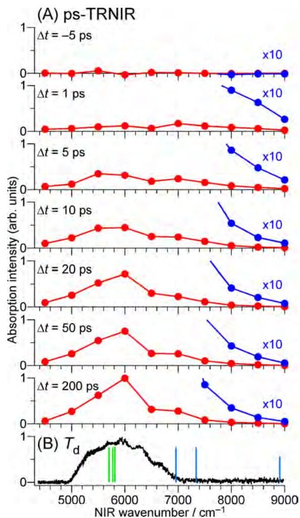
**Figure 4** (A) Picosecond time-resolved NIR spectra of PhOH-(NH<sub>3</sub>)<sub>5</sub> from  $\Delta t = -5$  to 200 ps. (B) The NIR spectrum measured by nanosecond lasers at  $\Delta t = 180$  ns. Green and blue bars represent theoretical spectra of the  $T_d$  and  $C_{3v}+1$  isomers, respectively. A common scale is used for vertical axes of time-resolved spectra to compare absorption intensities in different delay times.
