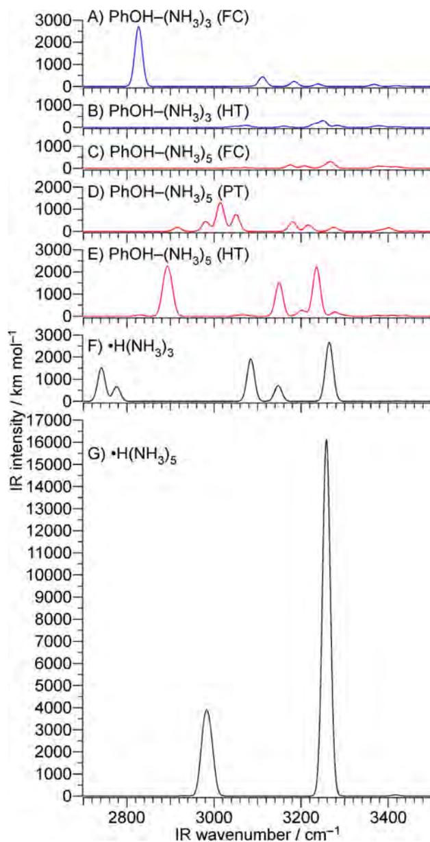
**Figure 9** A)–E) Theoretical IR spectra in the free NH stretching vibrational region of structures corresponding to A–E shown in Figure 8. F) and G) are IR spectra of the product radicals. A common vertical scale is used to all the spectra for the sake of comparison of the IR intensities.
