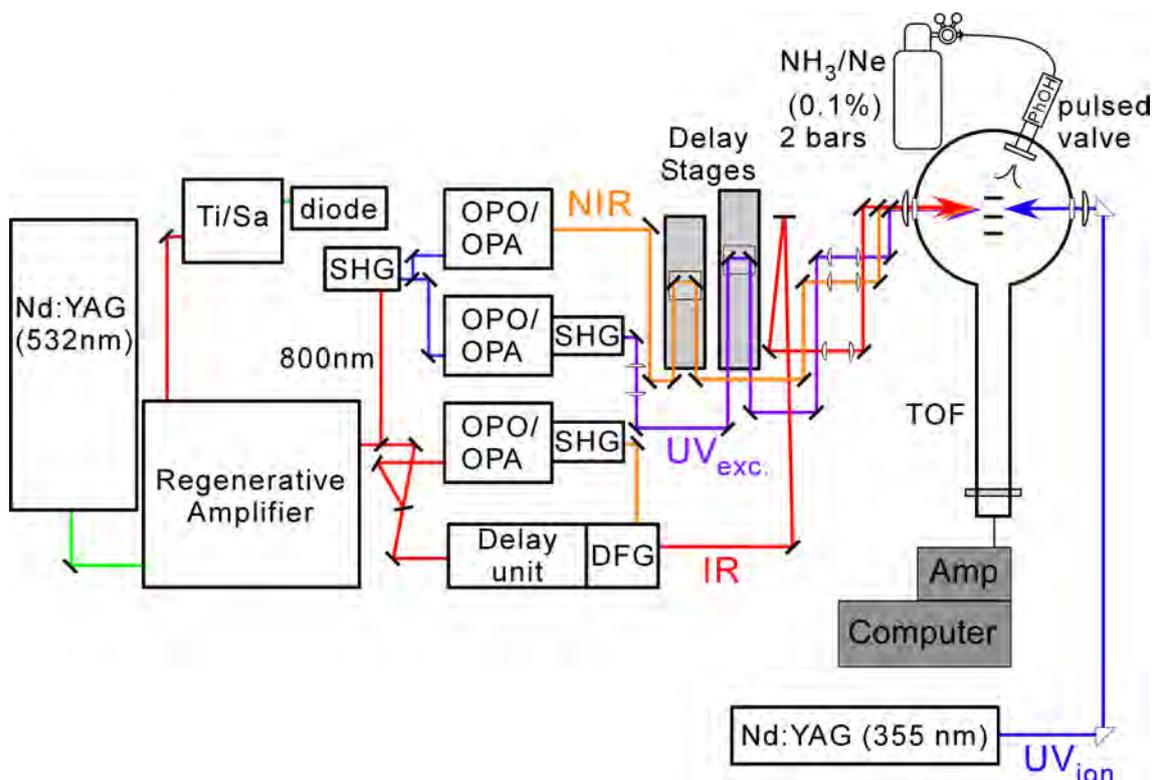
**Figure S1** A schematic diagram of the experimental setup of the picosecond time-resolved IR/NIR spectroscopy for PhOH-(NH<sub>3</sub>)<sub>n</sub> clusters.
