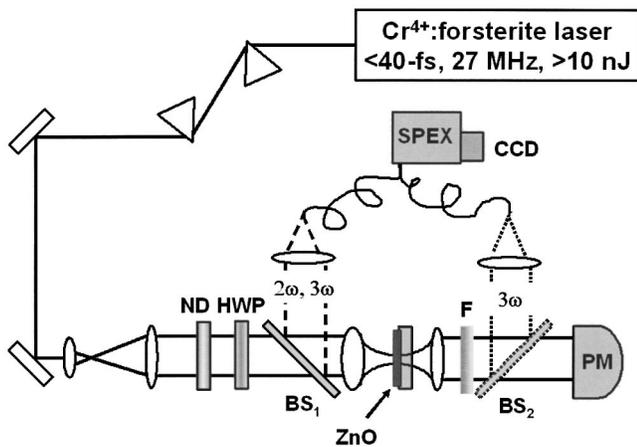
FIG. 1. Experimental setup for the THG. BS<sub>1,2</sub> are dichroic beamsplitters, ND is a neutral density filter wheel, F is a blue transmitting, near-IR absorbing filter, PM is a power meter, and HWP is a half-wave plate.
