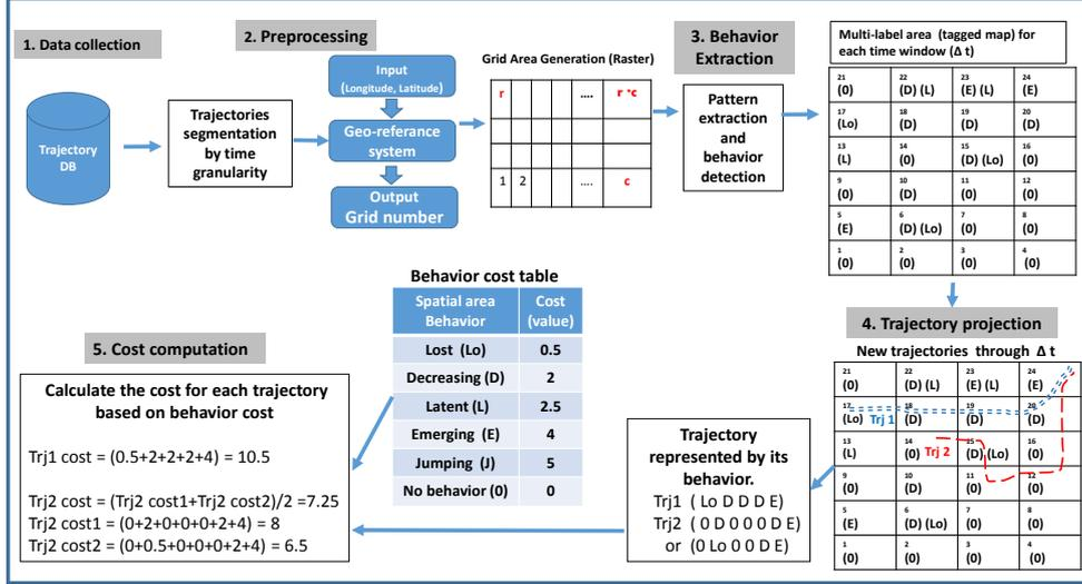
FIG. 1 – Overview of the proposed behavior based multi-label classification
