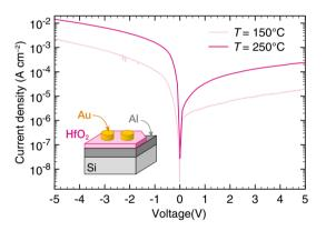
**Fig. 6** *j* vs. *U* curves for pour  $\text{HfO}_2$  layers grown at T = 150 and 250 °C. The scheme drawn on the plot depicts how the electrical measurements are performed: the back contact is established by the Al underlayer and the top contact by the Au dots
