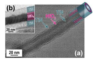
Fig. 7 a TEM micrograph of an MIM system (TiN/HfO<sub>2</sub>/TiN) grown by ALD within an AAM (the template has been etched in chromic acid to allow the observation). The number of cycles is 50/100/50, respectively. **b** TEM cross section of TiN/HfO<sub>2</sub>/TiN multilayers grown onto Si. The number of cycles is 250/500/250, respectively
