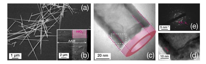
**Fig. 3 a** SEM top view of HfO<sub>2</sub> nanotubes after AAM dissolution in chromic acid. **b** SEM cross section of an AAM template after the ALD of HfO<sub>2</sub>. TEM image of a HfO<sub>2</sub> nanotube grown at T = 250 °C
