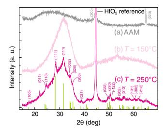
**Fig. 4** X-ray diffractograms of the AAM with indexed Al planes (**a**) and after ALD of  $HfO_2$  at  $150 \,^{\circ}C$  (**b**) and  $250 \,^{\circ}C$  with the monoclinic  $HfO_2$  indexed planes (**c**). Green marks indicate the expected peaks for a  $HfO_2$  powder diffractogram (PDF file 00-34-0104)
