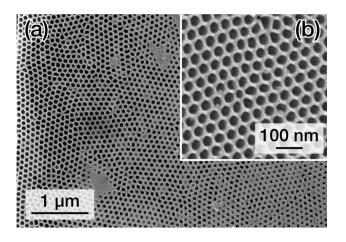
Fig. 2 a SEM top view of AAM grown in  $0.3 \,\text{M}\,\text{H}_2\text{C}_2\text{O}_4$  at 40 V. b High magnification view
