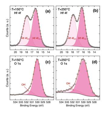
Fig. 5 Comparison of the XPS peaks of  $HfO_2$  layers grown at 150 and 250 °C. Hf 4f peaks are shown in **a** and **b** and O 1s peaks are shown on **c** and **d**. The temperatures of the ALD processes are indicated on the plots
