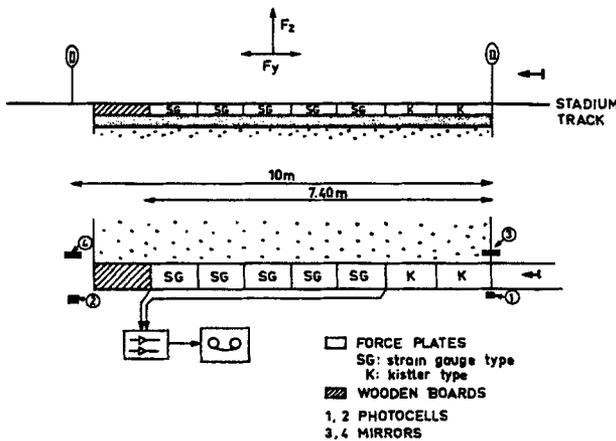
Fig. 1. Schematic description of the force platform and time-measuring device (photocells).
