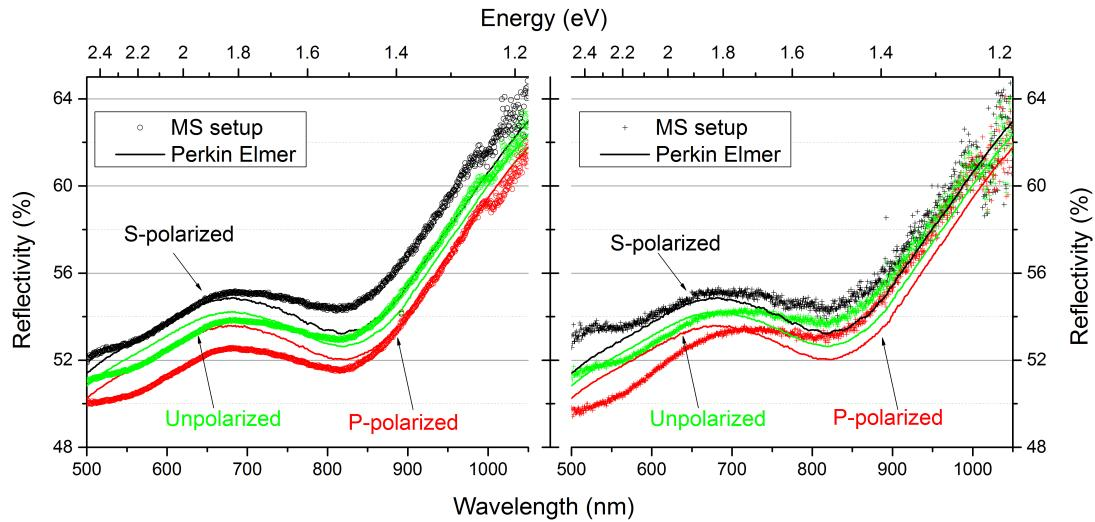
**Figure 2.** Reflectivity of tungsten for S-polarized (black), P-polarized (red), and unpolarized (green) light as a function of wavelength obtained with the MS setup described in section 2 (dots) and a Perkin Elmer spectrometer (solid lines). Spectra shown in left and right panels are performed without or with fused silica window in MS, respectively.
