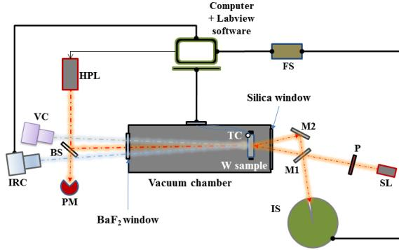
**Figure 1.** Schematic of the experimental setup: HPL, High Power Laser; BS, BeamSplitter; VC, Visible Camera; IRC, InfraRed Camera; PM, PowerMeter; TC, Thermocouple; M1 and M2, silver Mirrors; IS, Integrating Sphere; P, Polarizer; SL, Supercontinuum Laser.; FS, Fiber-optic Spectrometer
