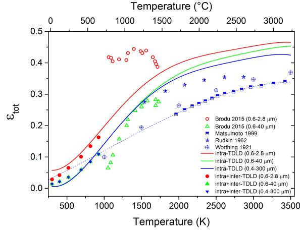
**Figure 9.** Calculated or measured total emissivity of tungsten from different references. Solid lines and full dots have been obtained for different spectral ranges through the intra-TDLD and the intra+inter-TDLD models, respectively. Blue dots are taken from Matsumoto *et al.*[26] (squares), Worthing[51] (pentagons) and Rudkin[52] (stars). Blue dashed curve is a fit of data from Matsumoto *et al.*[26] Open circles and triangles are taken from Brodu *et al.*[23]
