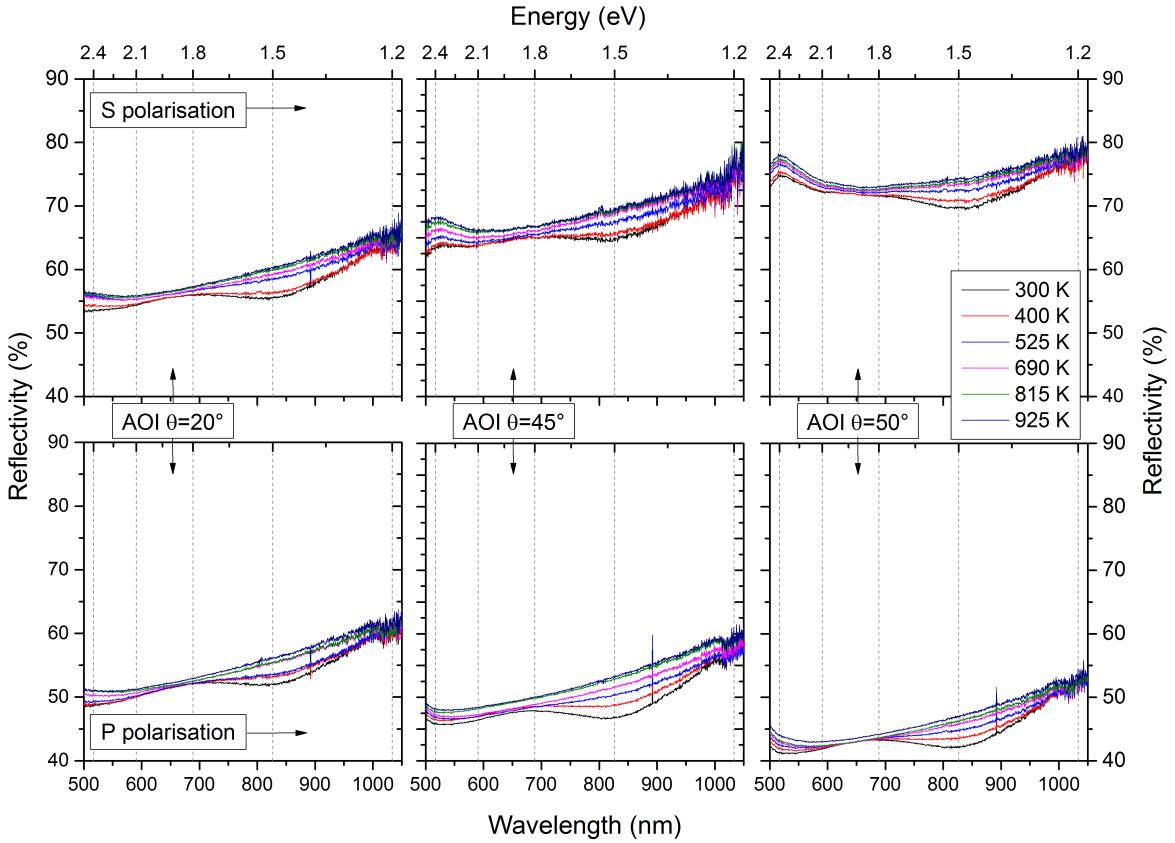
**Figure 3.** Reflectivity for tungsten of S (top panels) and P-polarized (bottom panels) light at six different temperatures (300, 400, 525, 690, 815, and 925 K) for three incidence angles (from left to right, 20, 45, and 50°) as a function of wavelength.
