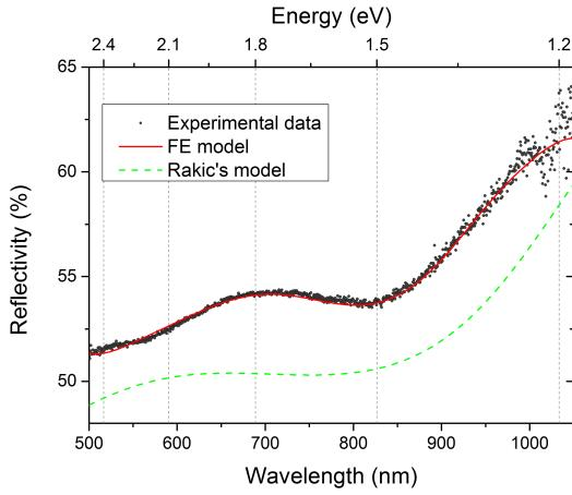
**Figure 6.** Experimental (dots) and theoretical (red line: Fresnel equations model; green dashed line: Rakic *et al.*[6]) reflectivity of tungsten at room temperature as a function of wavelength for unpolarized light at AOI=20°.
