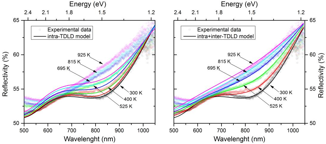
**Figure 8.** Measured and calculated reflectivity of unpolarized light at  $20^\circ$  of AOI. Lines are obtained by using the intra-TDLD model (left panel) and the intra+inter-TDLD model (right panel) for six different temperatures (300, 400, 525, 695, 815, and 925 K).
