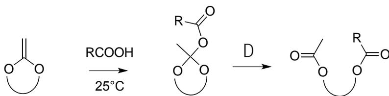
**Figure 67.** CKA rearrangement in presence of carboxylic acid.
