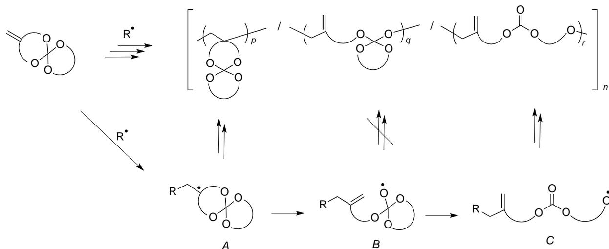
**Figure 11.** Polymerization mechanism of cyclic  $\beta$ -exo-methylene spiro-ortho-carbonates
