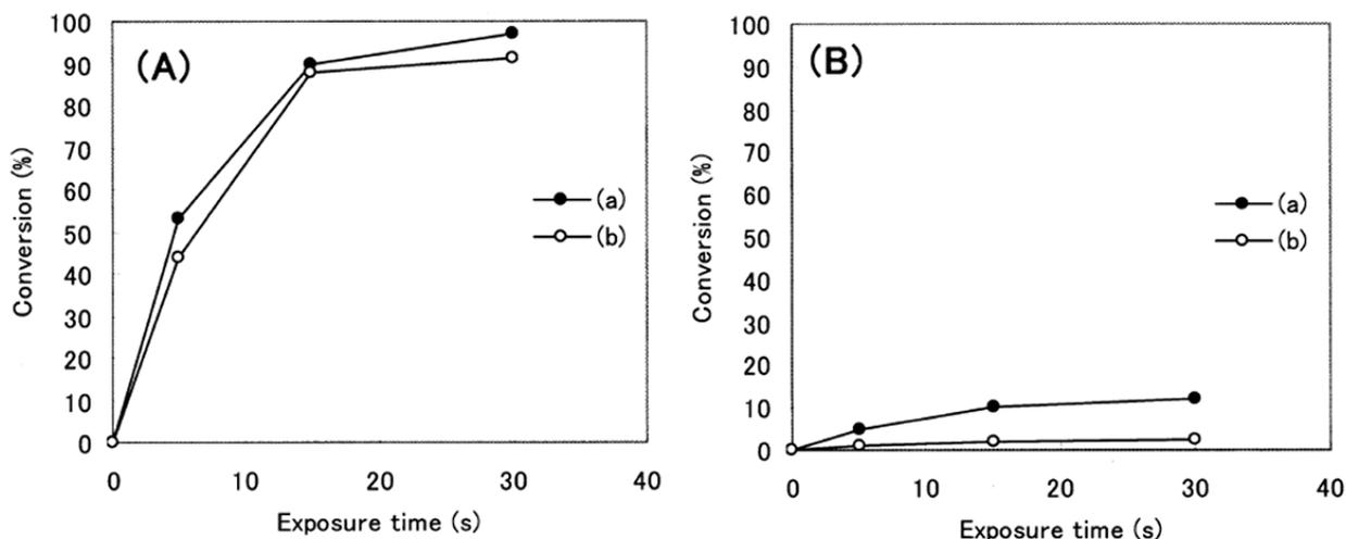
**Figure 35.** Conversion of monomer versus time plot for (A) CAS5 and (B) 2-ethylhexyl methacrylate under (a) nitrogen (b) air initiated with 2 mol% of lucirin TPO-L. Reproduced with permission from Ref. <sup>87</sup>. Copyright 2010 The Society of Photopolymer Science and Technology.
