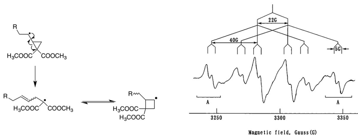
**Figure 52.** ESR spectrum observed during the polymerization of **VCP9** with MAIB at 60 °C in benzene. [VCP9] = 2.33 M; [MAIB] = 0.10 M; the modulation amplitude of 3.2 G was employed. Reproduced with permission from Ref. <sup>132</sup>. Copyright 2001 American Chemical Society.
