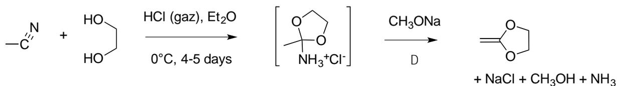
**Figure 62.** Synthesis of CKA according to Argade and coworkers.<sup>164</sup>
