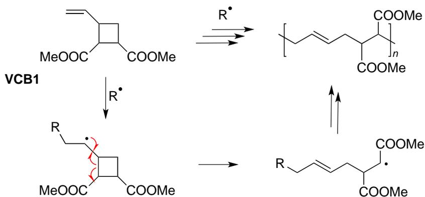
**Figure 8.** Mechanism of rROP of vinyl cyclobutane.
