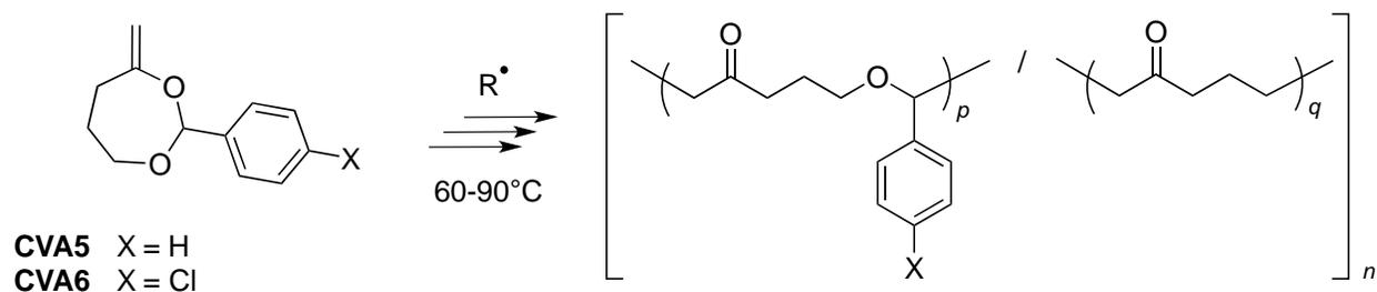
**Figure 24.** Polymerization of 4-methylene-2-phenyl-1,3-dioxepane (**CVA5**) and 4-methylene-2-(4-chlorophenyl)-1,3-dioxepane (**CVA6**).
