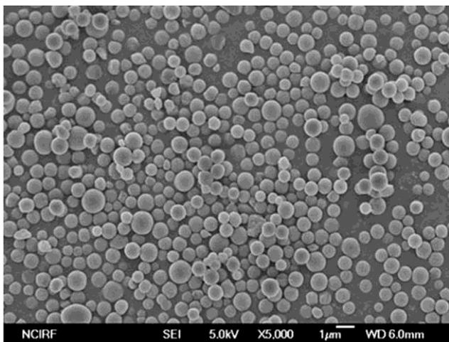
**Figure 122.** Field emission scanning electron microscopy (FE-SEM) images of copolymer particles with PHDFDMA (poly (3,3,4,4,5,5,6,6,7,7,8,8,9,9,10,10,10-heptafluorodecyl methacrylate) surfactant. Reproduced with permission from Ref. <sup>343</sup>. Copyright 2008 Springer.
