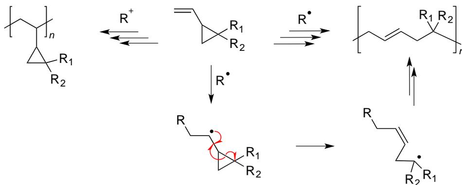
**Figure 6.** Vinyl cyclopropane radical and cationic polymerization mechanism.
