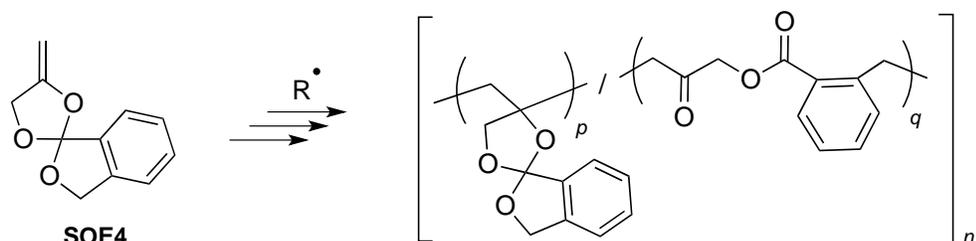
**Figure 14.** Polymerization of the cyclic spiro-ortho-ester **SOE4**.<sup>45</sup>
