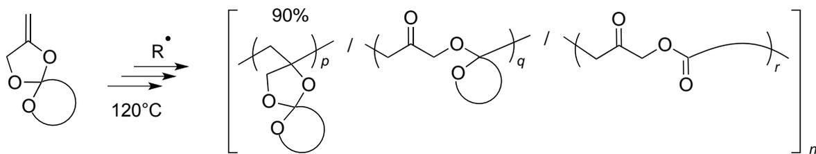
**Figure 15.** Polymerization of spiro-ortho-ester according to Ref. <sup>11</sup>.
