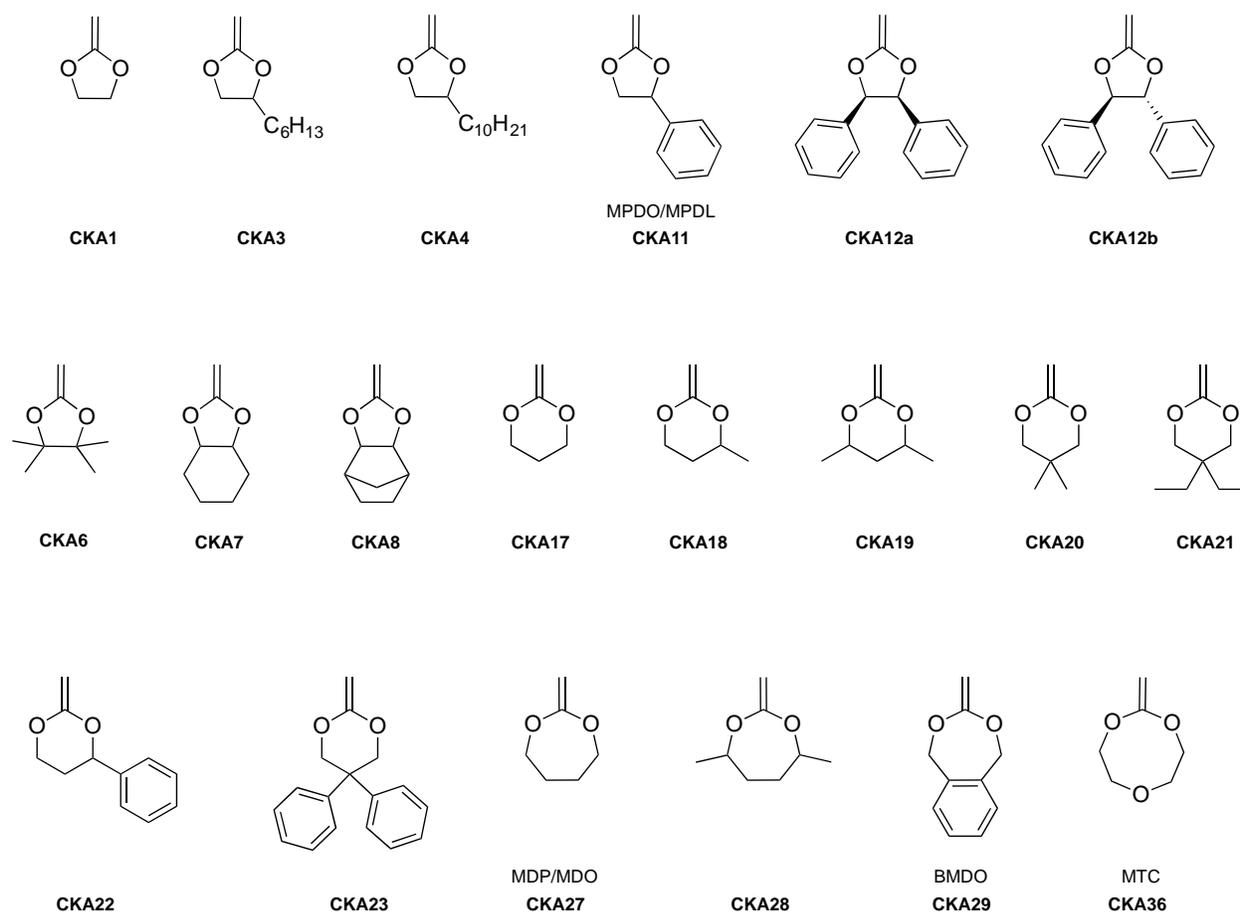
**Figure 72.** Principal CKA monomers studied in radical ring-opening polymerization.
