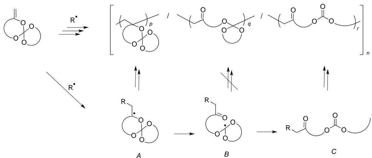
**Figure 12.** Polymerization mechanism of cyclic  $\alpha$ -exo-methylene spiro-ortho-carbonates.
