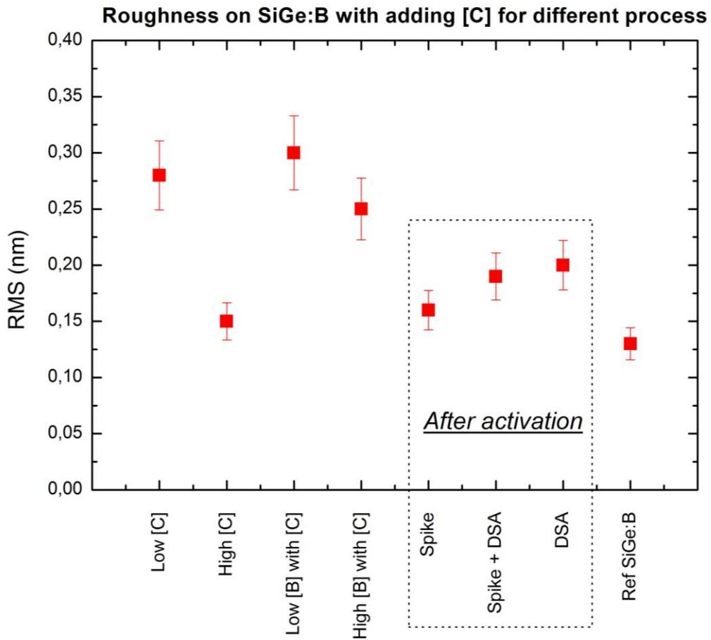
Figure 5. 30  $\mu\text{m} \times 30 \mu\text{m}$  atomic force microscopy images associated for different epitaxy process. RMS value on different SiGe:B for different epitaxy process and after activation. RMS value reference (no adding [C]) is 0.14 nm.
