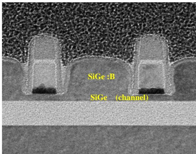
Figure 7. x-TEM image of selective  $\text{SiGe}:\text{B}$  with adding [C] epitaxial film grown on  $\text{Si}_{0.72}\text{Ge}_{0.28}$  channel on patterned wafer.
