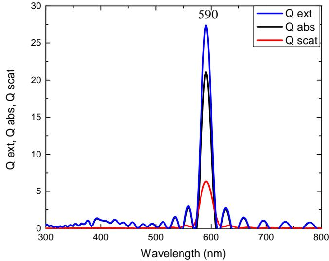
**Fig 2.** (a) Extinction efficiency of a nanoprism in water with different corner radius  $r$ , (b) maximum electric field enhancement for  $r=0$  nm and  $r=4$  nm. Radiation is normally incident along  $z$ , polarized along  $x$ . (c)  $Q_{ext}$ ,  $Q_{abs}$  and  $Q_{scat}$  for  $r=2$  nm.
