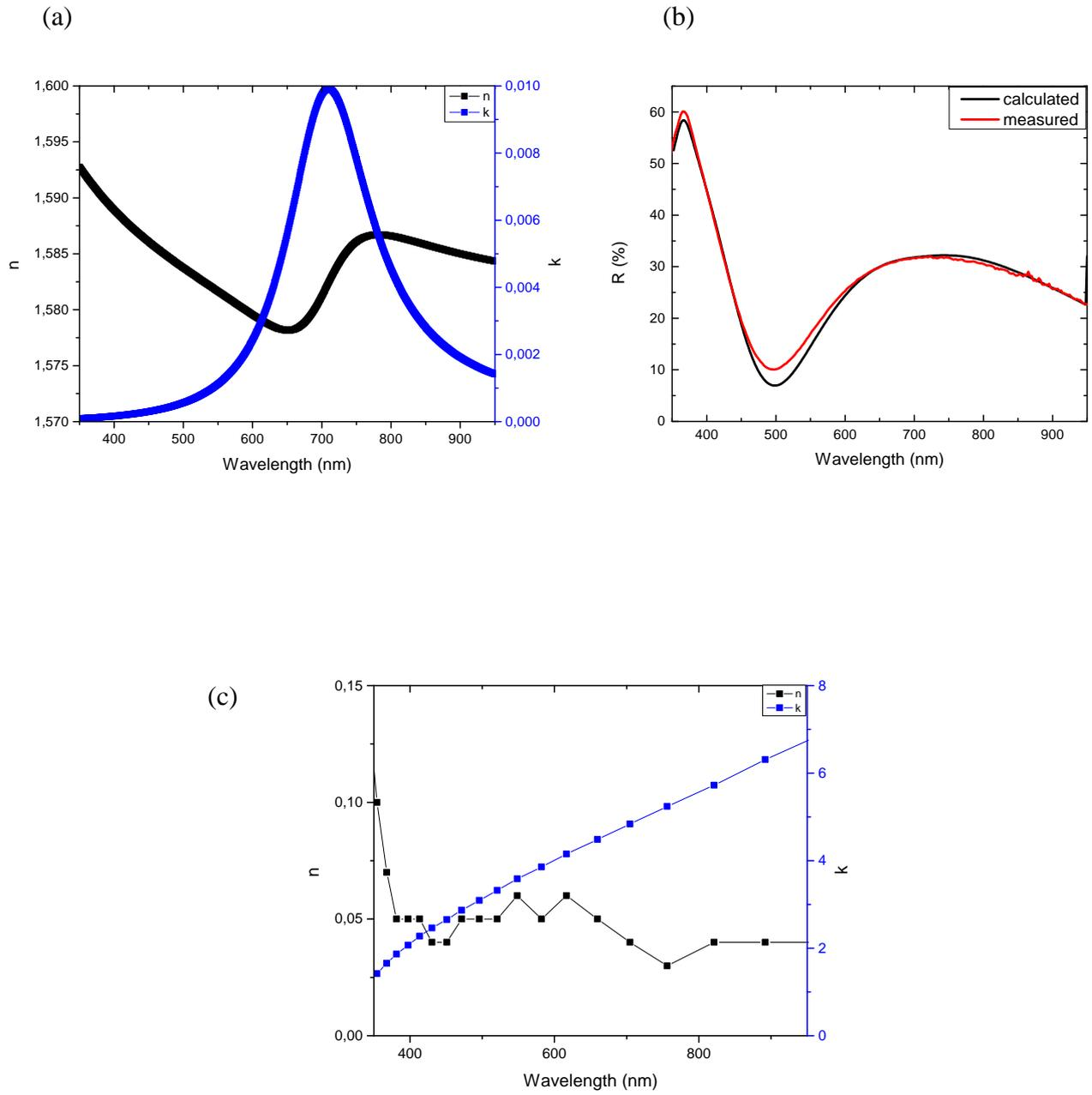
**Fig. 3** (a) Measured  $n$  and  $k$  of a heterogeneous PVP layer containing in average 25 nm edge size nanoprisms and (b) comparison of measured and by TMM calculated  $R$ , (c)  $n$  and  $k$  for bulk silver from Johnson and Christy<sup>11</sup> for comparison.
