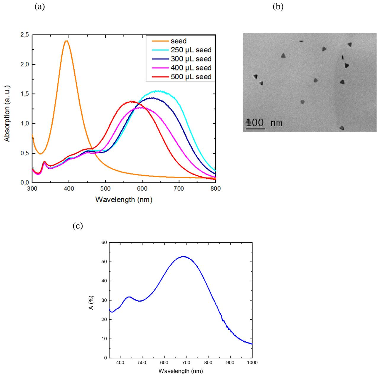
**Fig. 1** (a) Absorption spectra of colloidal solutions of the spherical seeds and differently sized nanoprisms resulting from adding various seed quantities in the second step of the synthesis, (b) TEM image of the produced nanoprisms, (c) absorption spectra of nanoprisms in PVP on glass.
