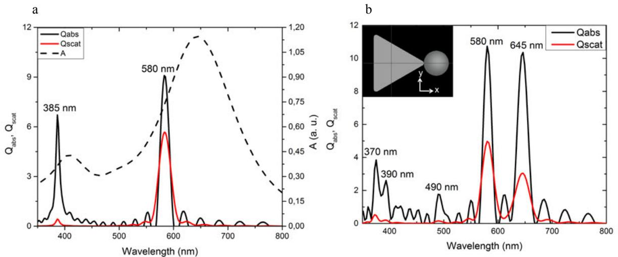
Fig. 3. Calculated  $Q_{abs}$  and  $Q_{scat}$  (a) for separated NP and the  $A$  of the colloidal solution, (b) for two NP system as depicted in insert.
