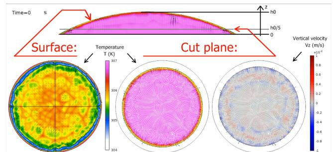
Figure 1 – 3D unsteady computations: thermal and velocity fields over the droplet surface and in a cut plane.
