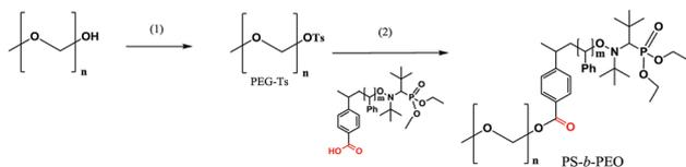
**Scheme 3** The reaction scheme for preparation of block co-polymers via the post-functionalisation approach. (1) Tosylation of PEG: a solution of PEG in pyridine and addition of TsCl at room temperature. (2) Grafting of polystyrene: addition of KOH into methanol with subsequent evaporation, addition of a solution of PEG-Ts to dimethylformamide, and heating for 80 h at 80 °C.
