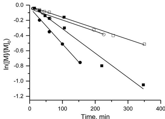
Fig. 5 Comparison of bulk polymerisation kinetics of styrene (squares) and 2-vinyl pyridine (circles) at 110 °C initiated with **3e** (filled symbols) or **3f** (open symbols). Solid lines show a linear fit of the data.
