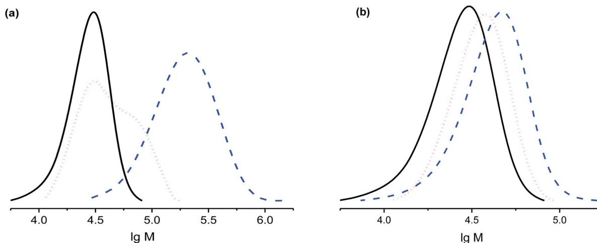
Fig. 8 GPC traces of re-initiation experiments with polystyrene prepared with **3e** as a macro-initiator (solid curve). (a) Re-initiation with styrene, at the monomer/macro-initiator ratio 0.5 g to 10 mg,  $T = 110\text{ }^{\circ}\text{C}$ , sampling at 0.5 h (red dotted curve) and 3 h (blue dashed curve). (b) Re-initiation with MMA, at the monomer/macro-initiator ratio 0.5 g to 10 mg,  $T = 80\text{ }^{\circ}\text{C}$ , sampling at 0.5 h (red dotted curve) and 1 h (blue dashed curve).
