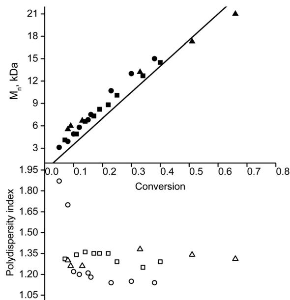
Fig. 2 Plots of molecular mass (filled symbols) and polydispersity index (PDI, open symbols) vs. conversion for bulk polymerisation of styrene at 110 °C initiated with **3d** (squares), **3e** (triangles) or **3g** (circles) at the monomer/initiator ratio of 350 : 1.
