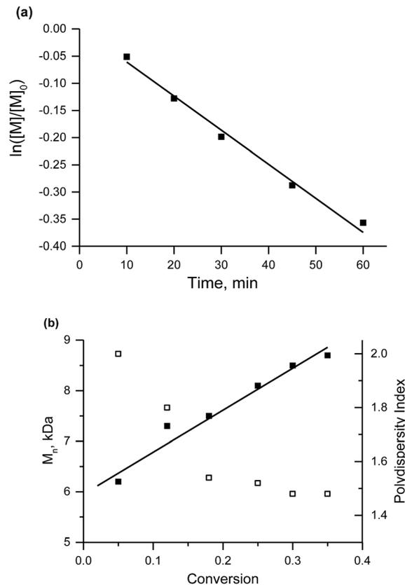
Fig. 6 The plot of  $\ln([M]/[M]_0)$  vs. time (a) and molecular mass vs. conversion (b) for co-polymerisation of methylmethacrylate with 2% of 2-vinyl pyridine in bulk initiated with **3e** alkoxyamine at 80 °C and the monomer-to-initiator ratio 350 to 1.
