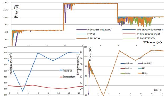
Figure 6: Simulation for change in irradiance and temperature.
