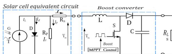
Figure 1: Equivalent circuit model of PV panel
