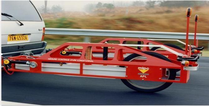
Fig. 7. Longitudinal Profile Analyser (APL in french)
