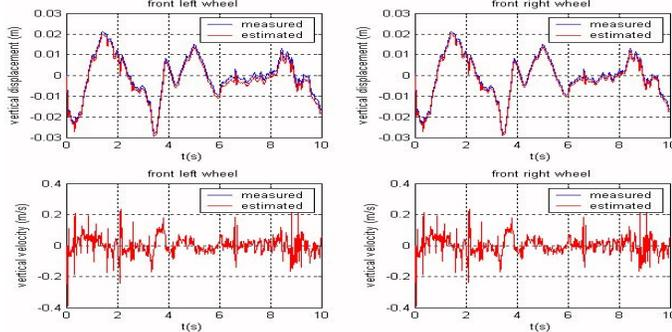
Fig. 8. Estimated and measured displacement of the wheels
