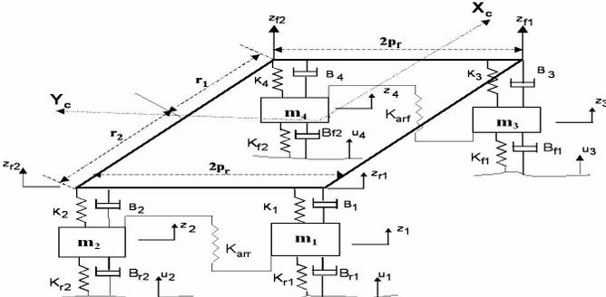
Fig. 3. Vehicle Model for estimation of road profile
