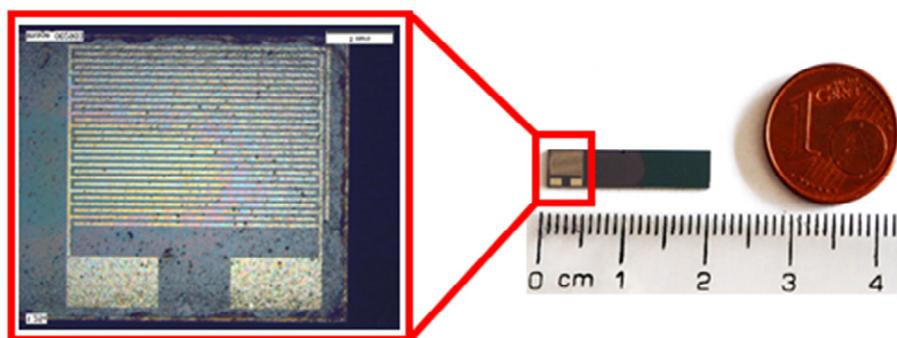
Fig. 1. Sensors fabricated on Si/SiO<sub>2</sub> based on AZO nanocrystals deposited by drop coating.
