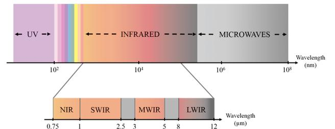
Fig. 3: Infrared wavelength in the electromagnetic spectrum.
