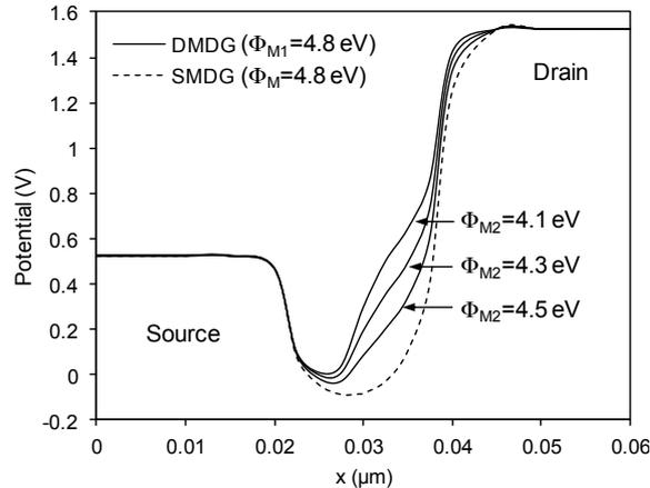
Fig. 2. Surface potential profile in SMDG and DMDG.
