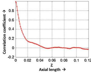
Fig. 4 Two point correlation for streamwise velocity
