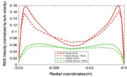
Fig. 5 Standard deviation of velocity for F2 case
