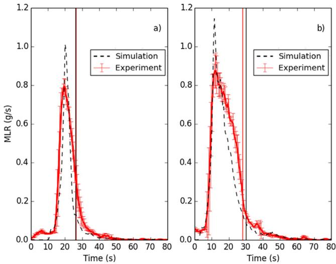
**Fig. 11.** Mass loss rates (MLR) at HF for different bulk densities (a) 23 kg/m<sup>3</sup> and (b) 40 kg/m<sup>3</sup>. Error bars: standard deviation. Vertical line: flameout time.
