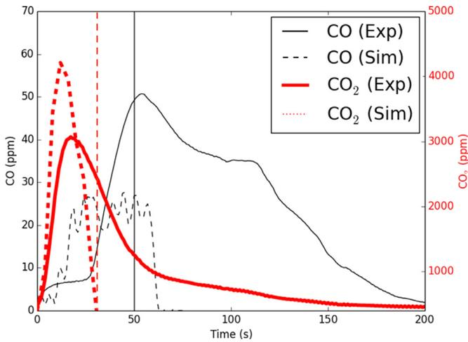
**Fig. 17.** Measured and simulated CO and CO<sub>2</sub> production (NF - 40 kg/m<sup>3</sup>). The vertical lines represent the experimental (red dashed) and the numerical (black solid) flameout times. Plots are shifted to have ignition at 0s. (For interpretation of the references to color in this figure legend, the reader is referred to the web version of this article).
