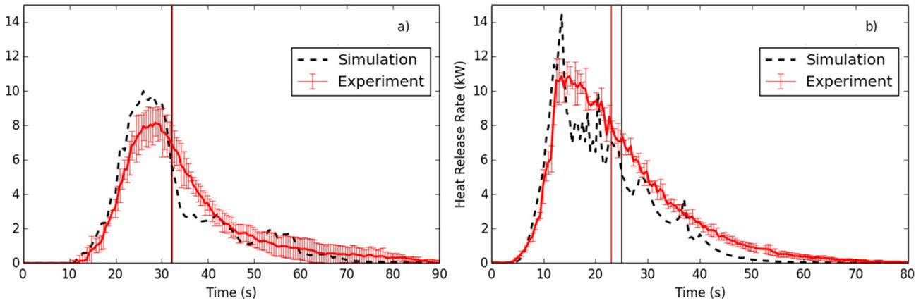
**Fig. 13.** Measured and simulated Heat Release Rates at HF for different bulk densities (a)  $23 \text{ kg/m}^3$  and (b)  $40 \text{ kg/m}^3$ . Error bars: standard deviation. Vertical line: flameout time.
