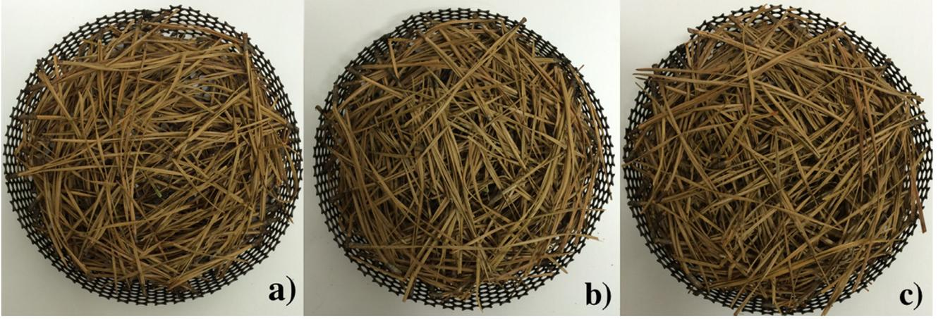
Fig. 2. Pitch pine needle samples with (a) 23 kg/m<sup>3</sup>; (b) 30 kg/m<sup>3</sup>; (c) 40 kg/m<sup>3</sup>.
