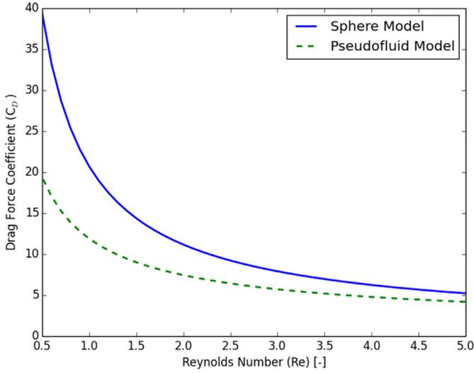
Fig. 4. Drag force coefficient estimation using different submodels.
