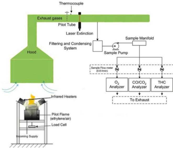
Fig.1. Overview of the Fire Propagation Apparatus (FPA).
