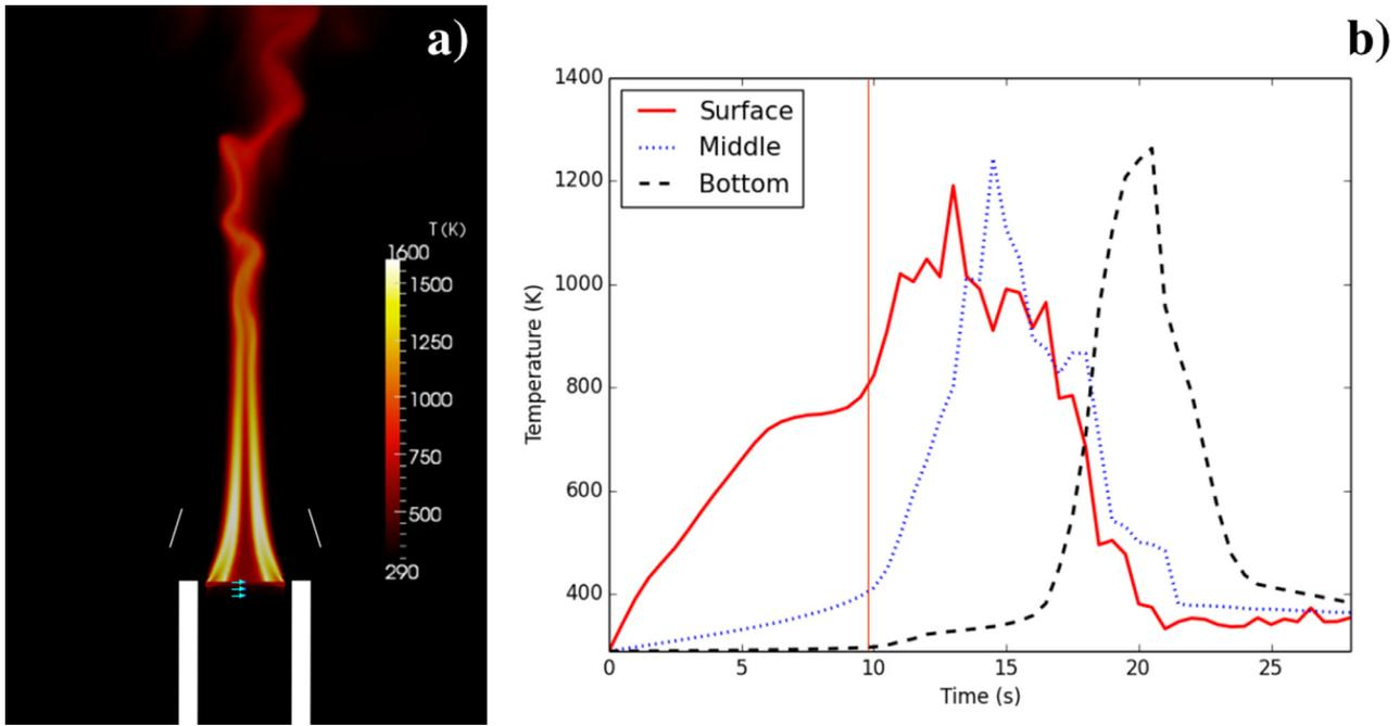
**Fig. 8.** (a) Temperature field during flaming (b) Simulated solid temperature at the top, middle and bottom of the sample corresponding to the three blue sampling points in (a), for HF and  $40 \text{ kg/m}^3$ . Vertical line marks ignition. (For interpretation of the references to color in this figure legend, the reader is referred to the web version of this article).
