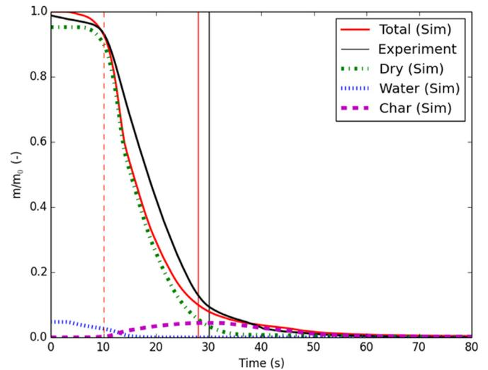
**Fig. 10.** Experimental and simulated mass loss, including simulated mass loss of dry, water, and char phases. Vertical dotted line corresponds to experimental and simulated ignition times. Solid vertical lines correspond to simulated and experimental flameout times respectively. (HF -  $40 \text{ kg/m}^3$ ).
