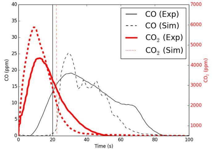
**Fig. 16.** Measured and simulated CO and CO<sub>2</sub> production (HF - 40 kg/m<sup>3</sup>). The vertical lines represent the experimental (red dashed) and the numerical (black solid) flameout times. Plots are shifted to have ignition at 0 s. (For interpretation of the references to color in this figure legend, the reader is referred to the web version of this article).
