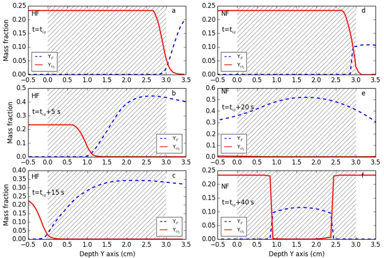
**Fig. 15.** Fuel and oxygen mass fractions along the vertical and at the center of the sample (hatched area) during flaming. Figures a, b, and c correspond to distributions at ignition, 5 s and 15 s, respectively for HF conditions. Figures d, e, and f correspond to distributions at ignition, 20 s and 40 s, respectively for NF conditions.
