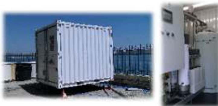
Figure 1. UF pilot plant [2 industrial modules 84m 2 , MWCO = 100kDa]
