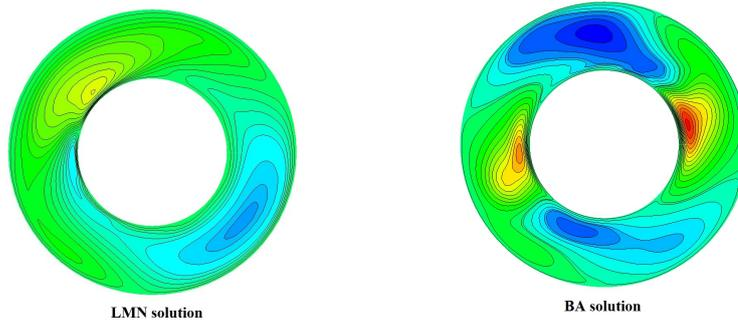
Figure 1: Iso-contours of radial velocity at mid-height of the cavity for  $Re = 1000$ ,  $Fr = 0.58$  ( $\Delta T = 24K$ ) and  $\mu = 0.35$ . Left: Low Mach number approximation (azimuthal wavenumber  $m = 1$ , frequency  $\omega/\Omega_i=0.54$ ). Right: Boussinesq approximation ( $m=2$ ,  $\omega/\Omega_i=1.12$ ).
