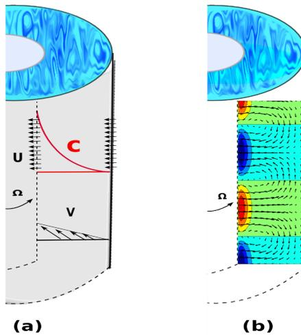
Figure 1: Figure of studied situation: a) Configuration and sketch of the base state ( $U, V$  : radial and azimuthal velocity components,  $C$  : concentration profile), b) Perturbation to this base state in a meridional plane.
