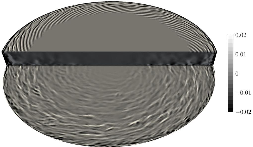
Figure 1: Instantaneous flow pattern in the whole cavity for  $Re = 4 \times 10^5$ . The stator is below. Iso-surfaces and iso-contours of the instantaneous axial velocity  $w$ . Three dimensional view. The rotor and stator boundary layers are shown for  $z = \pm 0.97H$ , respectively.
