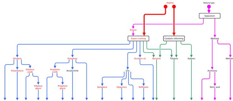
**Fig. 3.** Schematic of petrochemistry conversion pathways [6]
