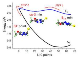
Figure 6 Energy profiles for the  $T_1$  and  $S_0$  states connecting the two  $T_1$  minima and the  $T_1/S_0$  crossing point for 6n-2tThy at CASPT2 level. The related key structures are indicated too.
