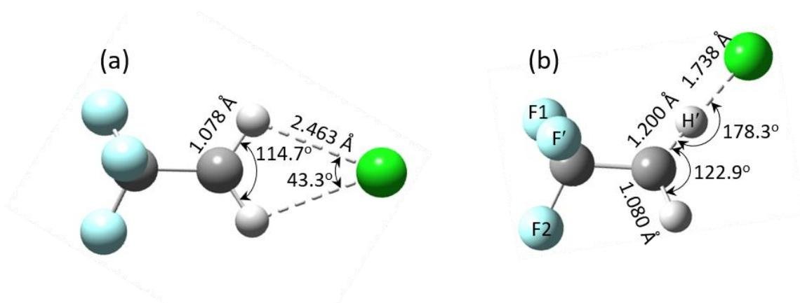
**Figure 3.** (a) Transition state resulting from the geometry optimization of the  $3^1A'$  state based on the relaxed scan shown in Figure 2; (b) Structure of the hydrogen-bonded ion pair obtained for the  $3^1A'$  state of the  $CF_3CH_2Cl$  molecule, computed at the MR-CISD/*valence* level with the B2 basis set. The main geometrical parameters are shown in the plot. F1 and F2 refer to the F atoms that are closer to the CCH' and CCH planes, respectively.
