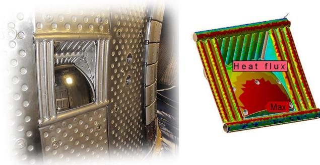
Fig. 3. Left: Mirror mounted in the inner wall of WEST - Right: calculated heat flux deposition pattern from plasma radiation (max = 130 kW/m<sup>2</sup>).
