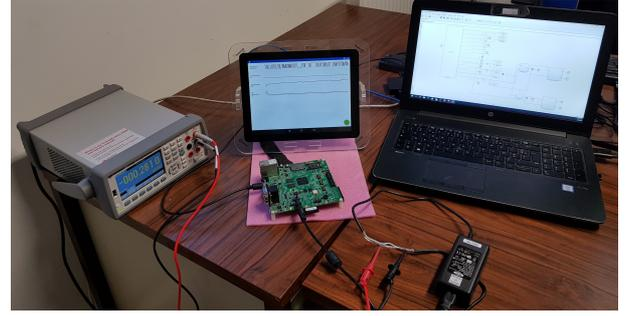
Figure 2: Overview of the application support including the development board, the display and the monitoring system.
