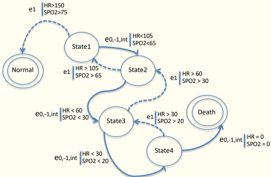
**Figure 11:** State-chart diagram modelling the new-born's behaviour according to the right or wrong execution of the ventilation gesture.  $e_{0,-1,int}$  is a shortened notation meaning that the degradation transition can be  $e_0$ ,  $e_{-1}$ , or  $e_{int}$ .
