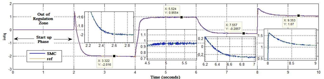
Fig.9. STATCOM  $q$ \_axes current variation as function of PCC voltage using SMC
