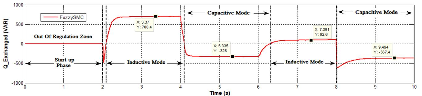
Fig. 8. The exchanged reactive power between STATCOM and the asynchronous wind turbine.
