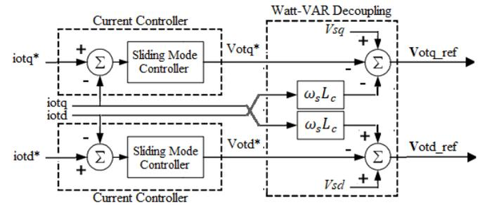
Fig. 3. Inner loop of current control
