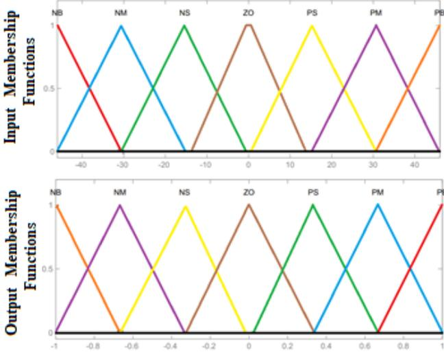
Fig. 5. Inputs and outputs membership functions of the SIFLC
