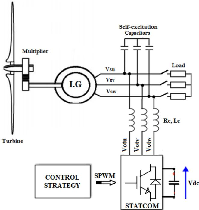
Fig. 1. Wind energy conversion system diagram
