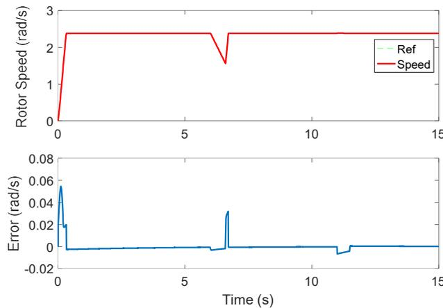
Fig. 5. Generator rotor speed response with ADRC.
