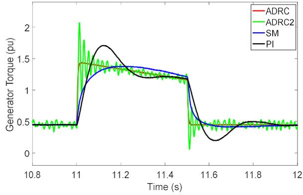
Fig. 9. Generator torque during turbine torque disturbance.
