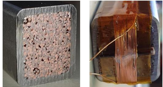
Fig. 1. MAG42-2, cross section of tested samples. 486 strands of 0.81 mm of diameter, with 324 of superconducting strands. Without (left) and with (right) the wound measurement pick-up coil.
