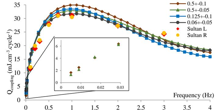
Fig. 3. Coupling losses on MAG42-3, similar to JT-60SA TF production cable. JOSEFA data comparison with SULTAN left and right leg. All curves are rescaled to  $B_m = 0,1T$ , the amplitude of SULTAN measurements. Included curves zoom in to confirm the good extrapolation.
