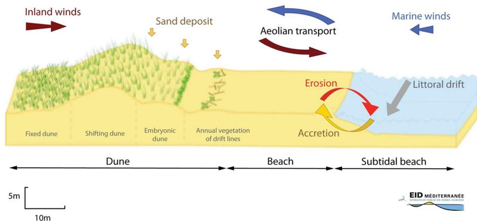
Figure 4.6 | Cross-section of a sandy dune system<sup>3</sup>
