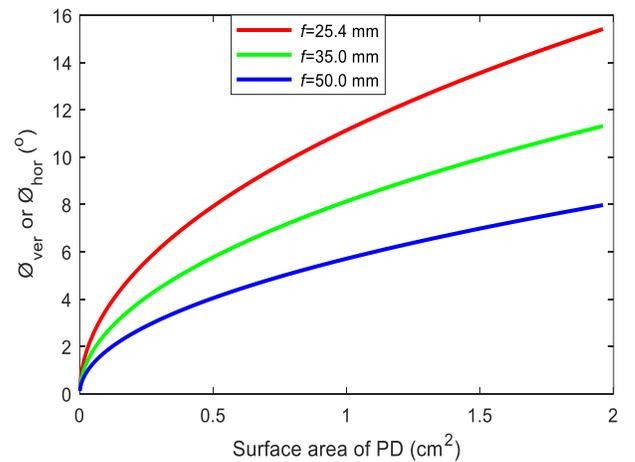
Fig. 6:  $\varnothing_{\text{hor}}$  or  $\varnothing_{\text{ver}}$  versus PD surface area for a range of  $f$
