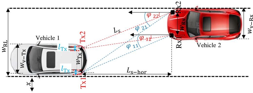
Fig. 3: VeLC configuration showing required horizontal AFOV
