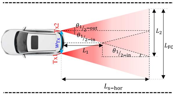
Fig. 7: Tx field of view (coverage diameter)
