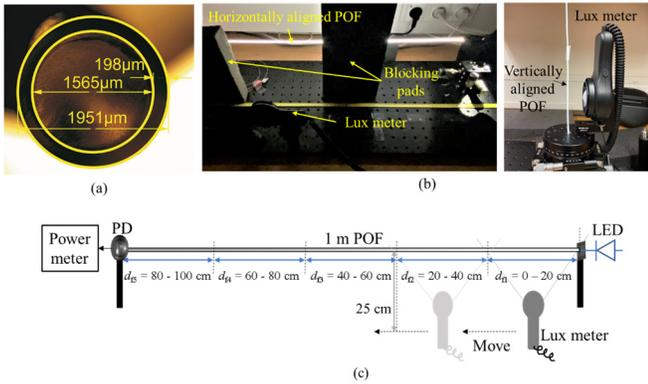
**Fig. 1.** (a) Microscope photograph of the used PMMA POF with measured core and cladding dimensions, including the cladding thickness, (b) Experiment setup for POF characterization of  $L-I-V$  and illumination pattern, and (c) characterization over  $d_f$ .
