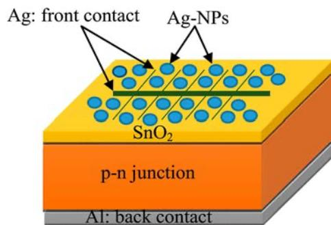
Figure 1 . Schematic representation of the experimental design.
