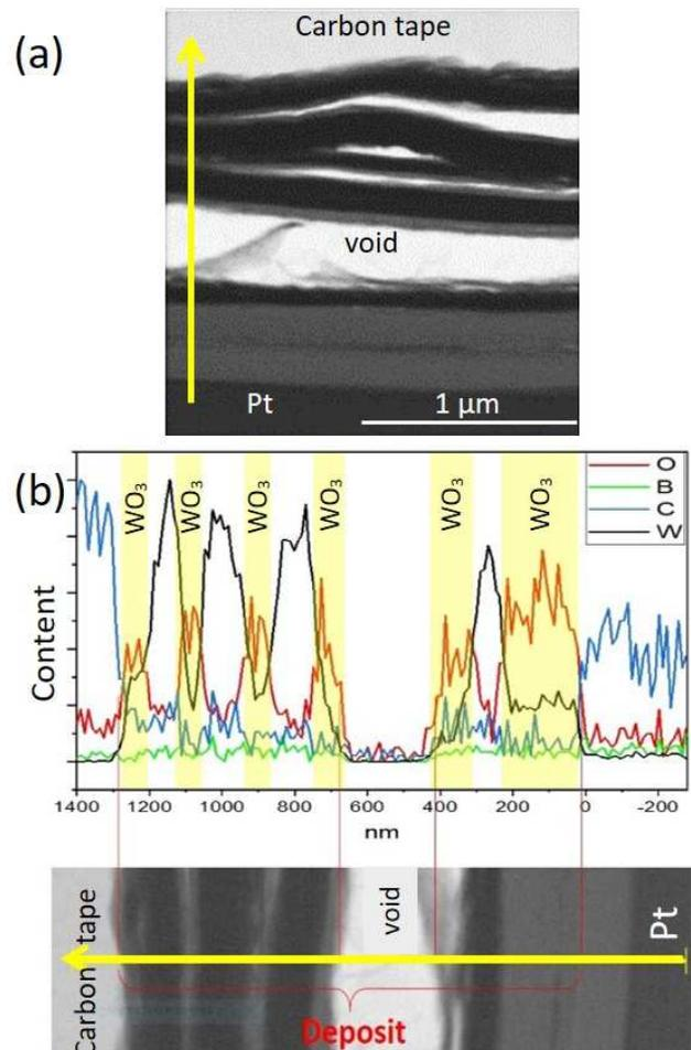
Figure 9: STEM bright field image (a) and (b) EDX depth profiling of FIB-thinned lamella extracted from MB 11 on WJKA004 after C3.
