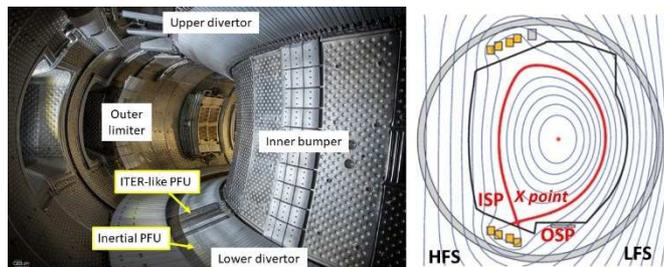
**Figure 1: Photograph of the WEST vessel during phase 1 operation (before the start of the C3 campaign in 2018), showing the lower divertor equipped with a mix of ITER like actively cooled bulk W PFU and inertial W coated PFU. Typical magnetic equilibrium in WEST, showing the inner and the outer strike points located on the same target is depicted in the right hand side of the figure.**
