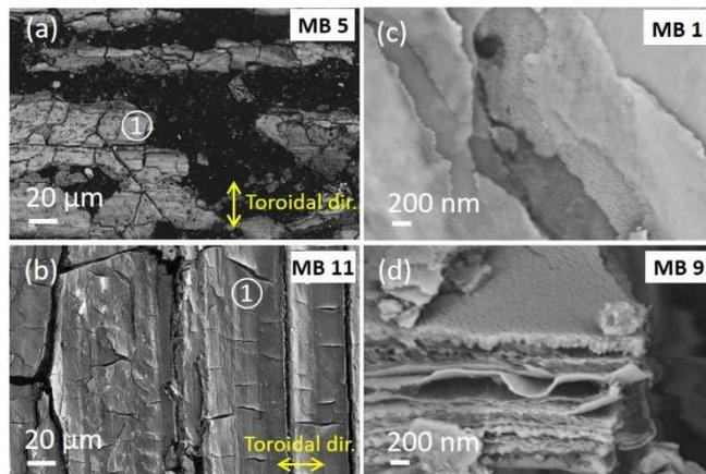
**Figure 4:** SEM images (BSE mode) showing the morphology of the deposits collected after the C3 campaign on (a) WERI002 MB 5 (b) WJKA004 MB 11 (SE mode for this image only). On the right hand side, high magnification images of WJKA004 (c) different textures found in the first layers of MB 1, (d) thin layers of different texture found in a deposit scrap observed by its section.
